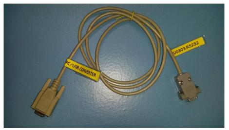
The side labeled with "SFU0303.RS232" mates to the connector of the SFU and the other one is directly compatible with the Com-Port at a PC.
