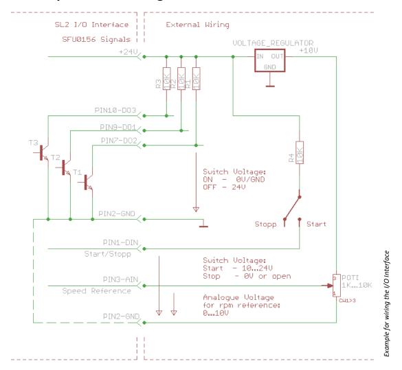
A successful start of the spindle the analogue voltage at PIN3 as reference for the duty speed hast be higher than the minimum voltage ( $\rightarrow$  5.2).
