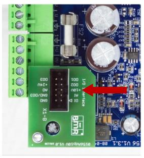
If a potentiometer (1-10KOhm) is connected between +10V and GND, a variable voltage can be set at the slider pin. If the slider is connected to AI (Pin3), the set value for the speed can be adjusted very easily according to the scaling of the analog input.
