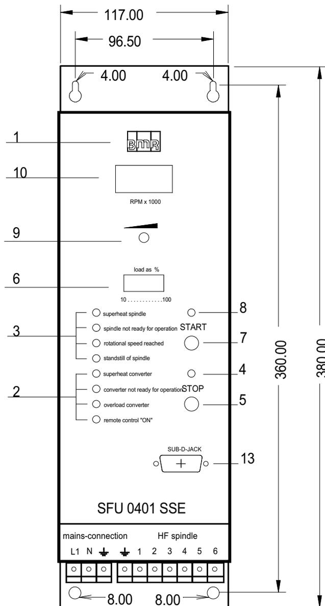
*front view of control cubicle configuration*
