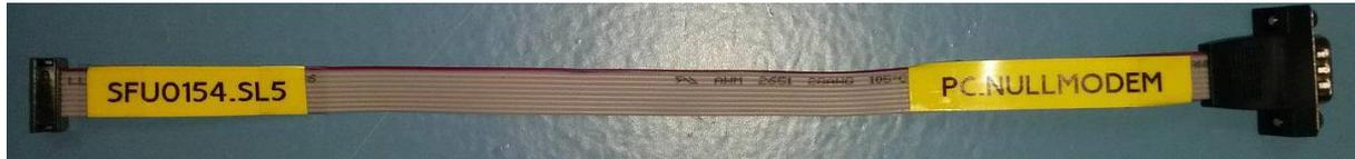
The side which is labeled with "Nullmodem" it has the standard RS232 PC COM-port pinout, so a Nullmodem can be used in conjunction with a PC
