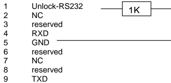
The resistor 1K from Pin1 to Pin 5 is required to unlock the interface
