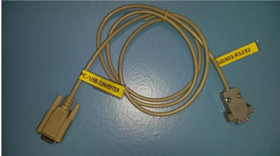
The side labeled with "SFU0303.RS232" mates to the connector of the SFU and the other one is directly compatible with the Com-Port at a PC.
